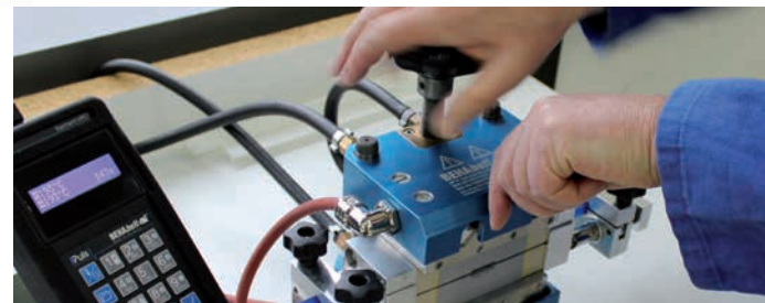
Turn the knob and close the press.
