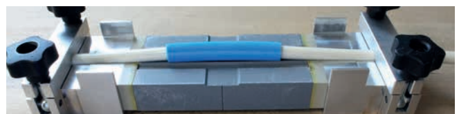
3. Positioning of the unwelded splice into the Mold
