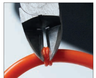
Remove welding bead with side cutter.
