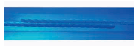
Overlap welding with reinforcement Overlap welding to reduce elongation and increase the belt tensile force.
