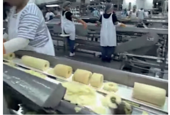
Conveying of cut pineapples on ESPOT belt with sealed edges.
