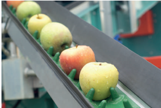
Special short finger profiles on a harvesting machine for thin skinned fruits (apple).
