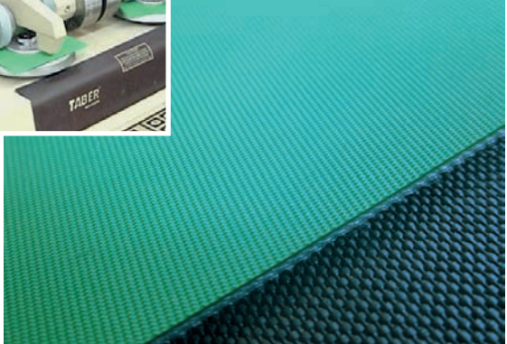
Y1 soft rough pattern and TABER comparative test machine.
