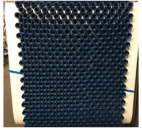
Depanner belts are used in bakeries to remove baked goods from metal pans after they come out of the oven. Depanner machines rapidly remove bread and buns from pans making bakeries more efficient than manual removal baked goods.
