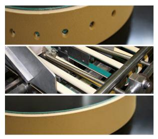
The setup of the feed section for any folder gluer is critical to success. Running a high quality feed belt improves gap consistency and produces a more square carton to improve your product quality.
