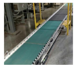
Motorized Driven Rollers (MDR) belts are utilized in distribution centers to minimize product gaps and maximize throughput. Precise product orientation and speed are required to ensure that the sortation process runs smoothly. Gapping, Metering, Merging sections all use endless elastic belts that take abuse daily while handling packages.
