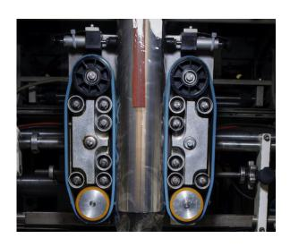
Vertical Form Fill and Seal belts are widely used for packaging snack foods in many industries. Designed to increase reliability and throughput, our VFFS belts are manufactured to multiple OEM specifications.
