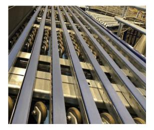
Sortation Conveyor belts frequently suffer from stretching, splice breakage, edge fraying and v-guide delamination.
