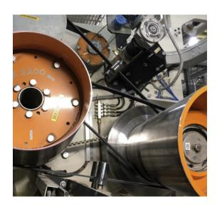
Standard cone drive belts experience speed inconsistencies, slippage, and early breakdown due to belt material and environmental conditions such as oil and grease.
