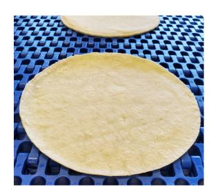
MIR offers solutions for all aspects of tortilla manufacturing. Our plastic modular belts are used in masa/dough handling, entering/exiting oven, bridge to cooling, multi-tiered cooling, counter-stacker and packaging.
