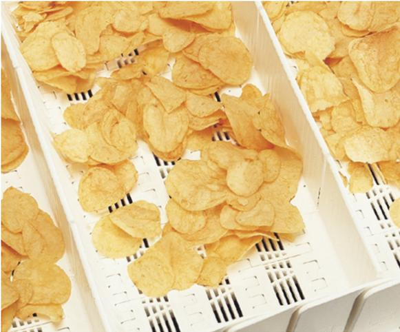
uni OPB 50mm pitch belt is designed for high performance with food products. Applications include cooking, blanching, seasoning and pasteurizing.
