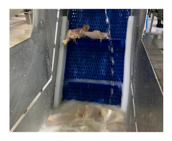
MPB 22% Open Blue Strong, easy-clean belt that reduces bacteria growth and supports heavy loads without breakage. MPB holds NSF/USDA approvals.
