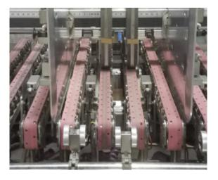
J&L Feed Belts are critical to properly infeeding the carton blanks into the folder gluer. Companies frequently experience delays due to extended belt delivery times by the OEM and other suppliers.
